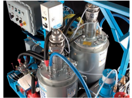
DUOMIX 333PFP -Zone 1- pneumatic agitators
