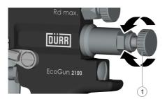
Fig. 3: Adjusting the withdrawal force
